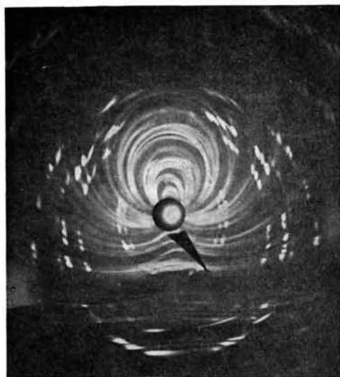
Fig. 8. Transmission pattern of mica rotated about the pole to its basal plane at a tilt angle of 16^\circ , downward.
